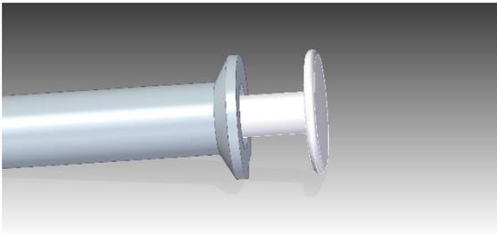
**WRONG** (insufficient) position of applicator plunger after the tablet should have been applied.
