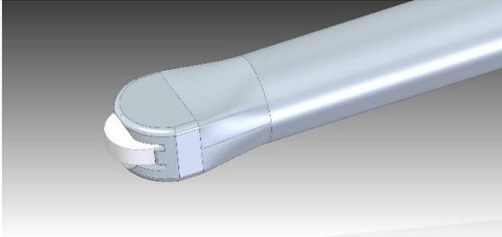
**WRONG** (insufficient) positioning of tablet in applicator.
